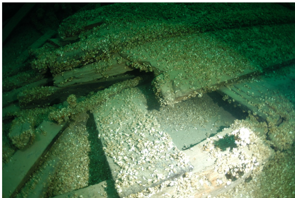
Figure 12. The port side turn of the bilge, aft of the collision damage. The chine log, sister chine log, and athwartship ceiling planks are visible. The bilge keelson is barely visible beneath the broken plank in the center of the photo.
