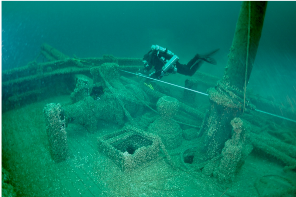
Figure 11. Forward deck including the windlass, capstan, forecastle scuttle, foremast, and bilge pump (aft of the foremast).
